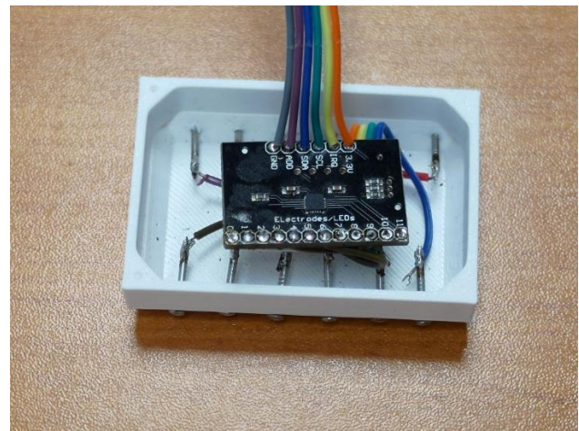
Fig. 1. Internal view of the rectangular prototype showing the MPR121 board and internal wiring.
