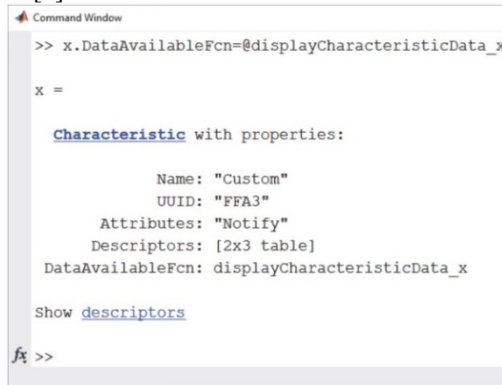
Fig. 1. Reading data from a sensor node via the MATLAB interface.
