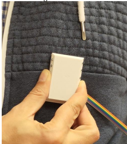
Fig. 2. A participant's hand performing the dual-side "grasp" on the rectangular prototype on lapel.
